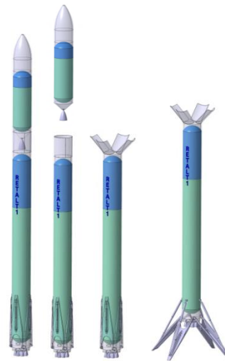
Fig. 4: RETALT1 (from left to right): launch, stage separation, first stage descent, first stage landing.
